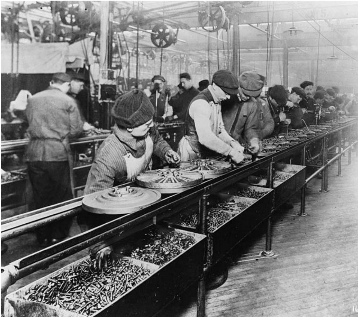
"Workers on the first moving assembly line put together magnetos and flywheels for 1913 Ford autos", Highland Park, Michigan.
